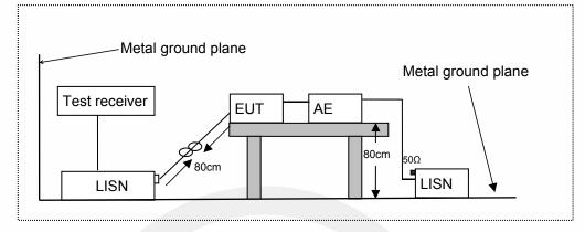
LISN: Line Impedance Stabilization Network AE: Associated equipment EUT: Equipment under test
